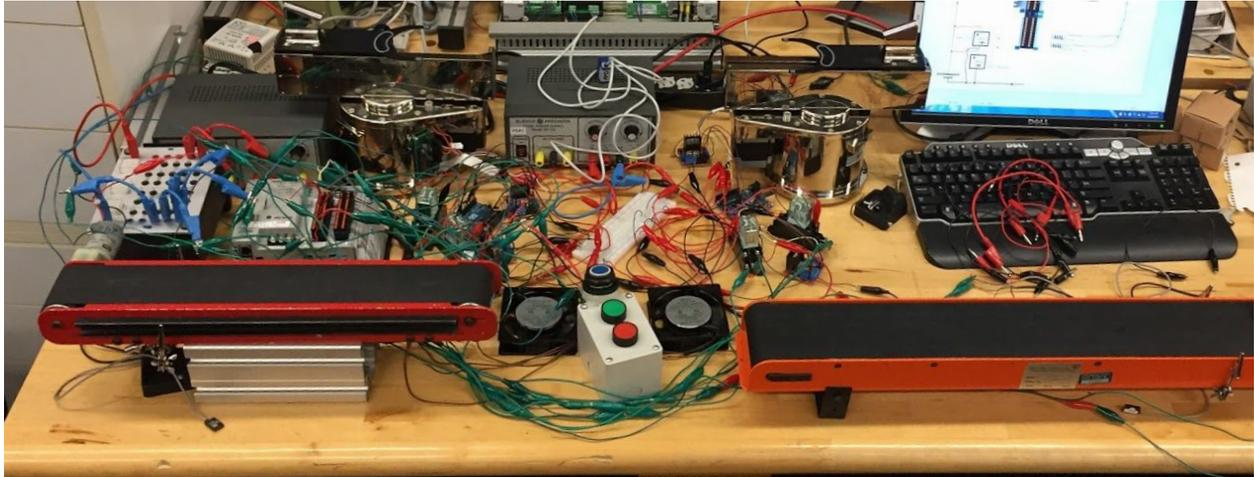
This next picture was a little more into the process. 120V fans were replaced with 24V fans, and I added extra relays to give reset functionality to the arduinos via the PLC.
